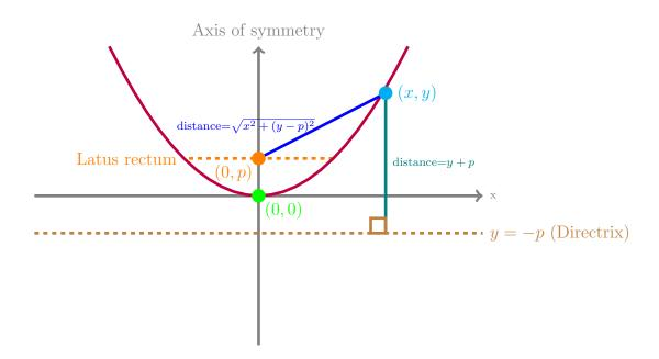
Note that the distance between the vertex, (0,0), and the focus and the distance between the vertex, (0,0), and the directrix are equal. That is why focus is denoted by (0,p) and directrix is denoted by y = -p. Now using these information we derive a closed form formula for the above parabola:
